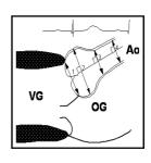
Measurements done according to the recommendations of the American Society of Cardiology (leading edge to leading edge, including the anterior wall and excluding the posterior wall). Left parasternal long-axis view (perpendicular to the long axis of the aorta, at end-diastole, averaging over at least 3 cycles).
